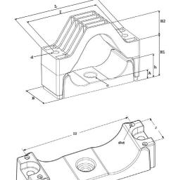
Initial torque for fastening fixing material : 5 - 8 Nm. (depends on cable manufacturer's prescription).
